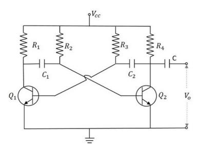
Two transistors named  $Q_1$  and  $Q_2$  are connected in feedback to one another. The collector of transistor  $Q_1$  is connected to the base of transistor  $Q_2$  through the capacitor  $C_1$  and vice versa. The emitters of both the transistors are connected to the ground. The collector load resistors  $R_1$  and  $R_4$  and the biasing resistors  $R_2$  and  $R_3$  are of equal values. The capacitors  $C_1$  and  $C_2$  are of equal values.
