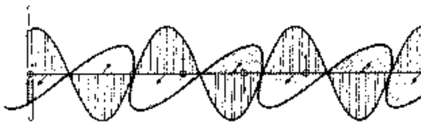
Figure 1-7 ► A harmonic electromagnetic field produced by an oscillating electric charge. The arrows without attached charges show the direction in which the north pole of a magnet would be attracted. The magnetic field is oriented perpendicular to the electric field.
